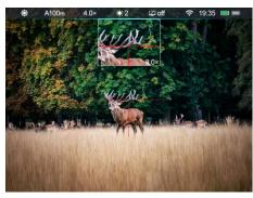
• On the home screen, press and hold the **image mode button (6)** to enable or disable PIP.
