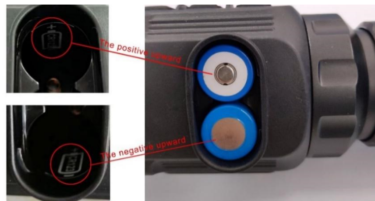
Fig. 8-1 Schematic diagram of battery installation
